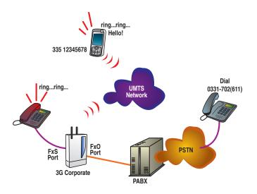
The voice applications of 3G Corporate allow its use as sole gateway in the most performing PABXs where the Internet connectivity is often required to take advantage of all the VoIP functions and Systems Messaging.
